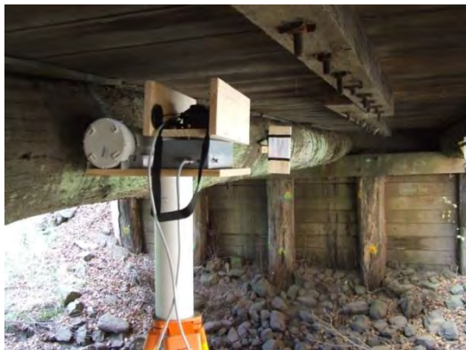
Figure 8: Optical source, high speed camera and graduated chart target
