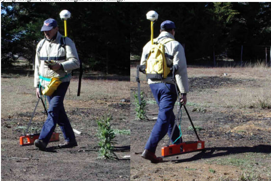
Figure 1 Author carrying EM-GPS over dispersal field, front and rear views
